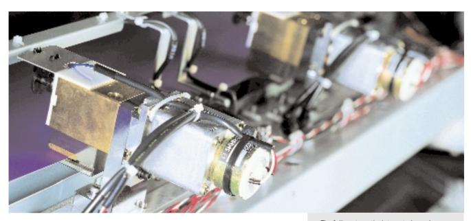
The fully automatic, integrated punch maximizes register accuracy and cuts press makeready times.
